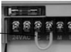
Replace with the two wires from the rain sensor into these terminals, polarity NOT required. Move the rain sensor switch on the fascia to “ON”.
