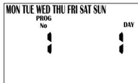
To turn Monday off press the **-** button. To turn it back on press the **+** button. To advance to the next day and set it use the **▶** button, the display will then flash Tue and Day 2. Use **+** or **-** to turn days ON or OFF and advance to the next day using **▶**. Remember to set all 7 days ON or OFF.
