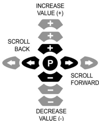
The **P** is used to select different programs. Each push on this button will increment one program number.
