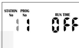
**NOTE:** This means that station 1 of program 1 has no run time programmed in it. The controller has permanent memory so when the device is first used there will be no run times set. Unlike other controllers, when there is a power failure, even if the battery is not installed, the programmed values will be restored to the unit.
